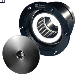
Recommended torque setting for the lock ring is 7Nm for M6 set screws and 35Nm for M10. This assumes stainless steel 304/A2 cup point set screw, made to DIN916/ISO4029, fitted to a dry, ungreased thread. It is recommended to pre-drill the stock at set screw locations to ensure a durable lock ring fit.
