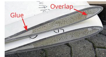
Due to the high pressure foam filling system, the foam is guaranteed present in all areas of the blade so no air pockets can be present. Also visible is the large overlap at the front and the huge glue contact area at the aft side of the rudder blade.
