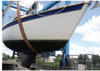
Boat hull after being in the water for 2 years with the Sonihull system.
