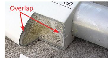
A unique feature of Jefa Rudders is the overlapping parts of the blades. This feature substantially strengthens the blade integrity, making it nearly impossible to split. Traditionally the rudder halves are glued heads on together, allowing only a very small contact area which causes the blade to split easily.
