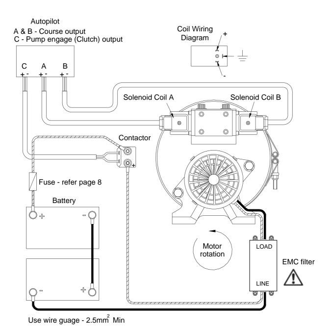
Attach leads to contactor as shown
